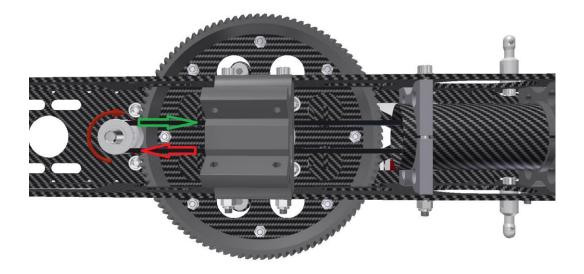
Guide the belt through the two clamping flanges without twisting further. At the same time slide also the tail boom into the two clamping flanges. In the picture the red arrow signifies the working strand of the belt and the green arrow signifies the relaxed strand. Push the boom forward until it almost touches the large gear so you can put the belt over the small pulley.
