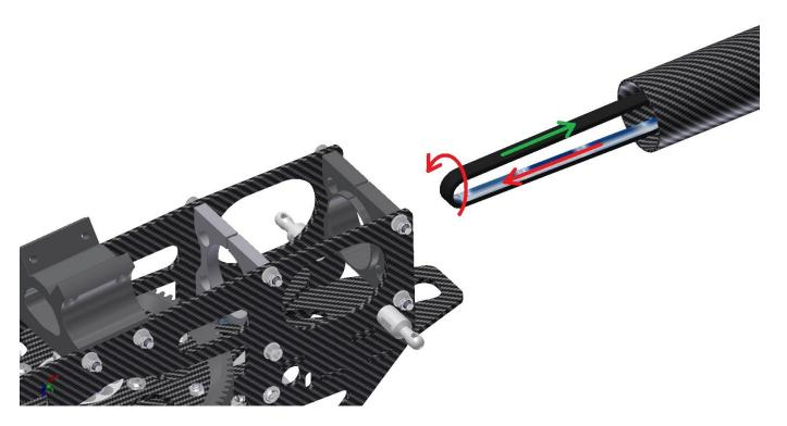
Turn the core mechanic and tail boom upside down then pull the belt toward the front out of the tail boom and align it in such a manner, that it runs straight without being twisted.
