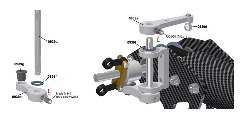
(left picture above) The bushing 0939g will be pressed from above into the lower bell crank 0939e. The shaft 0939c will also be slide into the hole from above and fixed at the flat surface area with a M3x4 grub screw. The shaft should look outside the bell crank by about 1,5mm to the bottom.
