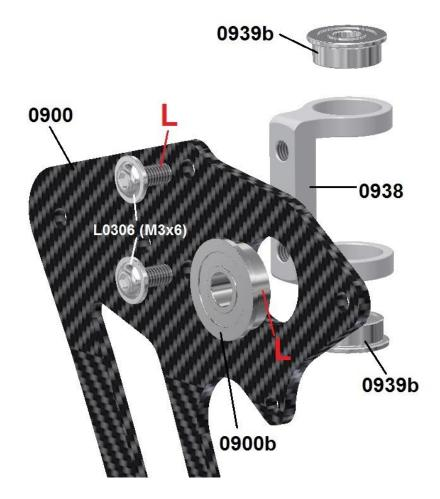
In the picture left you can see the preparation of the vertical fin plate which will be mounted later on the right side.
