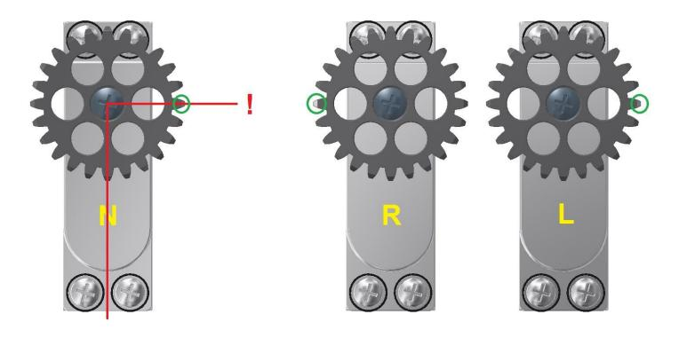
Now mount a servo gear 0640 on each swash plate servo.
