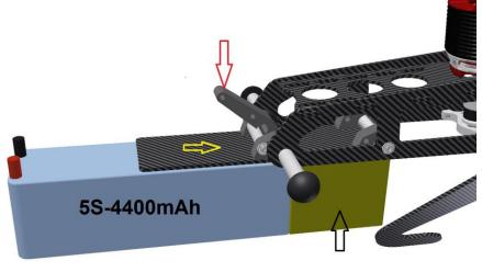
To lock the battery holder, push it with its hooks onto the silicone rubbers of the distance bolts (yellow arrow).
