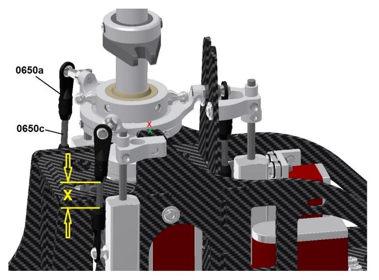
The three control rods between the gear racks and the swashplate has to be pre-assembled so that the distance (yellow X) is the same.
