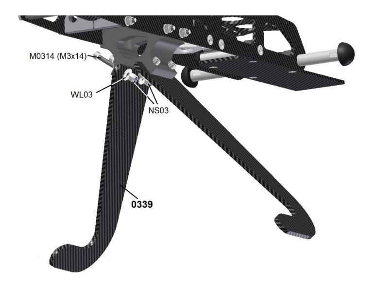
The 3mm thick CFK-skid plates 0339 are mounted on the skid holder as shown in the picture above.
