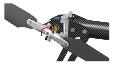
Attention! Keep in mind that the tail blades of the **TSDF** rotate in the opposite direction to most of the other existing model helicopters. If you observe the tail blades from the right side respective to the forward flight direction, they rotate clockwise. I have done this with all my helicopters ever since the beginning.
