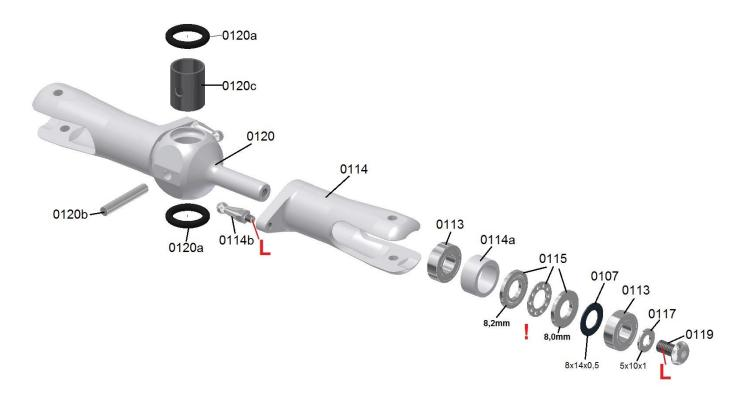
First, the blade grips will be equipped with the respective bearings.
