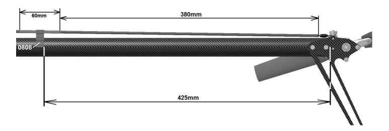
Before fitting the push rod, the approx. 60mm long shrink tube 0831c must be shrunk onto the push rod.
