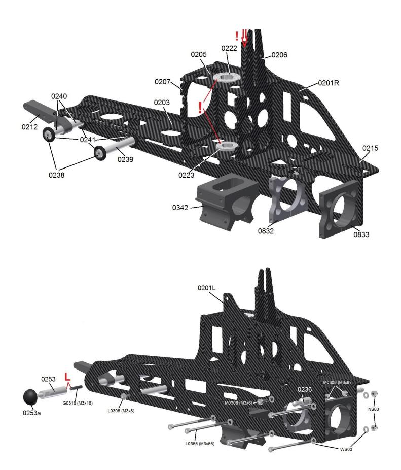
The chassis of the **TDSF** is plugged together and only glued to the individual latches within the chassis with a few drops of superglue. In order to avoid mistakes when plugging together and to check whether everything fits, we have already assembled the individual plates and <u>provisionally fixed them at a few points</u>.
