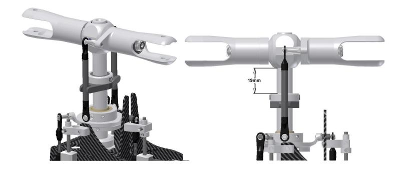
The control rods 0121a / b / c already prepared in "Chapter 1" are attached to the ball ends.
