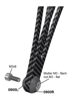
Press the ends of the two vertical fin plates together and screw them with the two plastic caps 0900L and 0900R.
