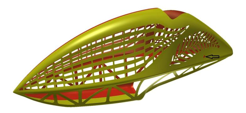
Note: The canopy is not as damageable as it looks because it is very flexible due to the many cutouts.
