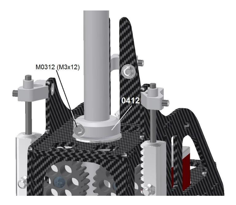
Mount the clamping ring 0412 on the rotor shaft.
