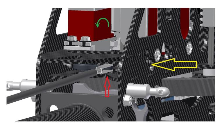
Now hang in the clevis into the lever of the tail servo with a distance of approx. 13mm to the servo shaft axis. The chassis side plate has a hole (yellow arrow) on the side, through which you can insert a screwdriver to carefully spread the fork head.
