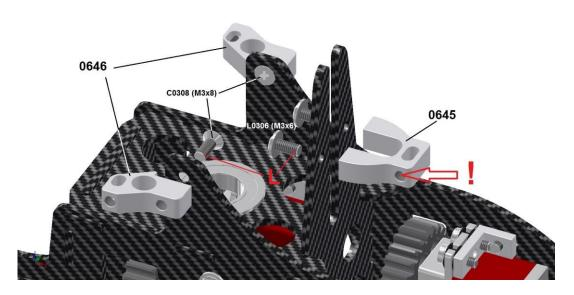
The two rack guide axle holders 0646 for the aileron servos are already mounted by us, because it is a little difficult to tighten the screw after gluing the chassis. May be they have to be aligned a little bit later.
