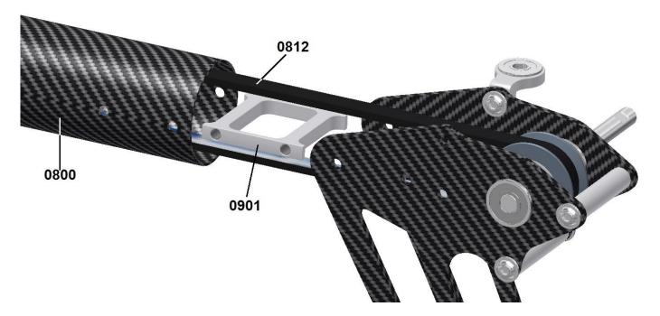
Pull the tail belt 0812 through the tail boom 0800 by using a long wire hook or a cord. Position the fixation insert 0901 between the two strings of the belt and position it in the tail boom aligning the threated holes with the holes of the tail boom.
