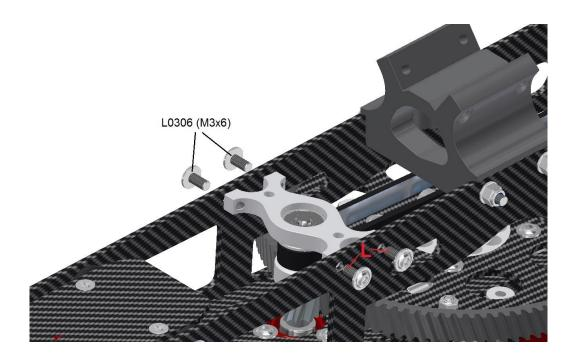
Finally, the four M3x6 lens head screws L0306 are alternately screwed stepwise with some Loctite and tightened well.
