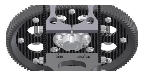
The flange is screwed to the rotor shaft with the M4x20 hex socket screw 0419 and an M4 stop nut.
