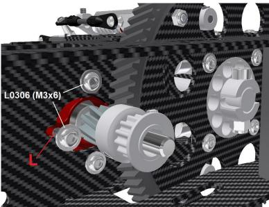
The bottom plate of the chassis has an elongated cut out, so that the motor can be easily inserted completed with the pinion.
