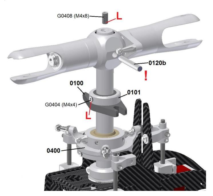
Slide the swashplate 0400 onto the rotor shaft so that the special ball stud with the sliding sleeve fits into the slot of the rear vertical stiffener plate.
