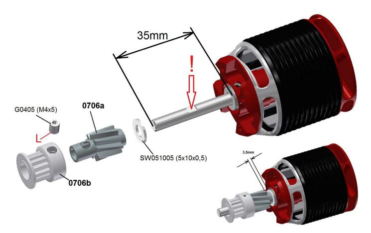
The motor must have a 5mm diameter shaft with a minimum length of 35mm measured from the motor bearing flange. Also a small approximately 0.4mm deep flattening in the middle with a width of 4 to 5mm is needed. In the case that only a shaft with a flattening over the entire length is present, this can also be used. It is important that there is a flattening in the area of the grub screw after sliding the pinion on the shaft.
