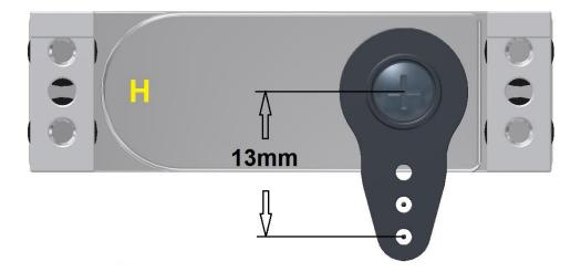
At the tail servo a standard servo lever (see drawing) is mounted, which has a bore on a radius of approx. 13mm.
