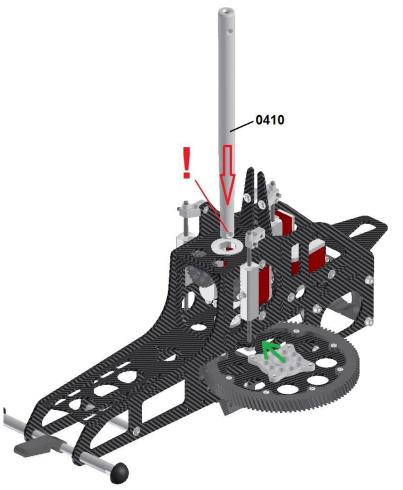
The gearwheel is pushed into the mechanics from the side until the hole of the flange aligns with the lower main rotor shaft bearing (green arrow).
