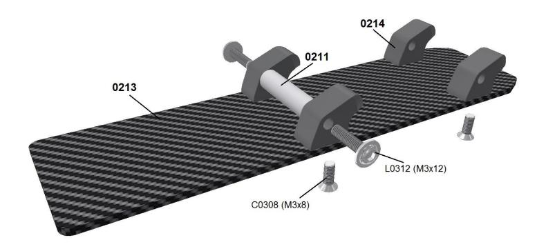
Fix the hooks 0214 with M3x8 counter sunk screws C0308 to the plate 0213.
