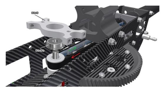
The flange bearing 0840b is pressed into support bearing plate 0840 as shown in the picture above. Then the bearing plate is slid onto the motor shaft from below until the lateral M3 threaded holes with the oblong holes in the chassis are at the same height without jamming the plate.
