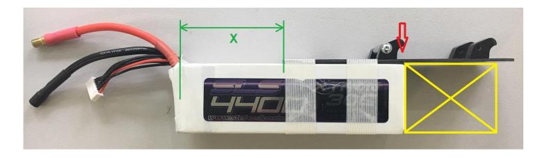
The picture above shows examples for the fixation of a 5S - battery to the respective battery trays.
