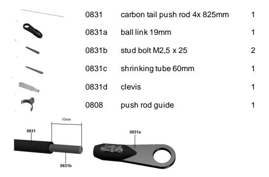
Glue the thread rods 0831b with thin superglue into both sides of the push rod 0831. 10 to 12mm of the thread should protrude on each side.
