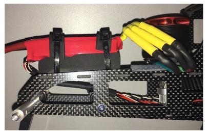
Unfortunately the Kolibri-controller is only smooth on the upper side, where the cooling plate is mounted under the shrink tube.
