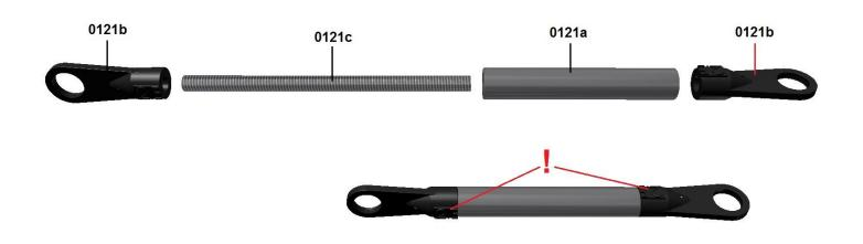
Mount the rod as shown in the picture above. Position the ball link in line to prevent damage.
