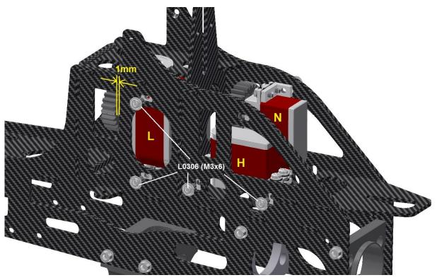
The servos are mounted in the chassis using M3x6 pan head screws as per drawing (use Loctite).
