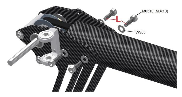
The unit will be screwed with four M4x10 screws M0310 and four washers WS03 to the end of the tail boom. Secure the screws with Loctite and tighten them well stepwise and alternating.
