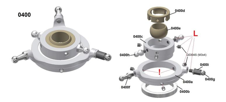
The swash plate will generally be delivered finally assembled. In case of a damage the swashplate can be disassembled partly.
