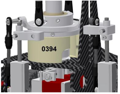
For fine tuning of the swashplate servo neutral position you can use the swashplate gauge 0394 (see picture above). For better visibility, the left chassis plate is not drawn.
